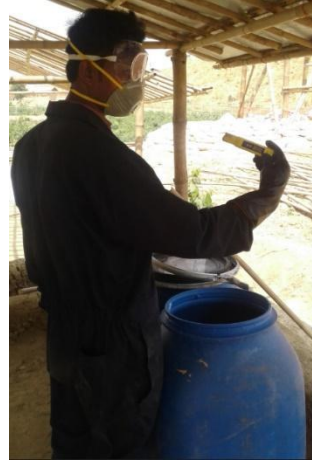
Lime treatment (pH measurement)
