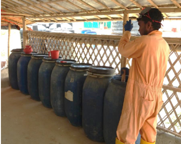
Bucket lime treatment
