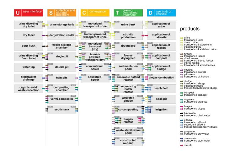
Figure 3.6: Overview of the sanitation technologies, products and functional groups (FGs) used in the example application in Nepal. Notes: (i) Storage (S) may also include (partial) treatment; (ii) Treatment (T) technologies may be applicable on-site (no transport required) or offsite; (iii) the model can also include non-toilet sources which allows the system boundaries to be extended (water tap, stormwater drainage, organic solid waste collection).
