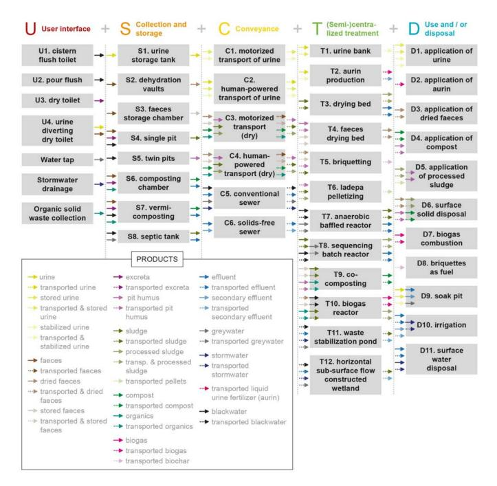
Figure 4.6: Overview of the set of sanitation technologies currently available in the technology library for five functional groups. Each box represents a technology. The arrows represent the input and output products. So far only toilet sources are implemented, although greywater, stormwater, and organic waste sources can also be considered by the model.
