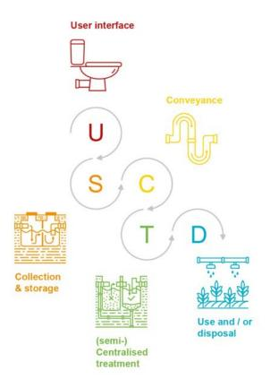
Figure 1.3: A Sanitation System is a context-specific series of technologies and services for the management of human wastes (or resources), from the point of generation to the point of reuse or disposal. This includes five functional groups: the user interface (U), the collection and storage (S), conveyance (C), treatment (T), and final reuse or disposal (D). Sources: (Maurer et al., 2012; Spuhler et al., 2018; Tilley et al., 2014b; Zurbrügg et al., 2009).
