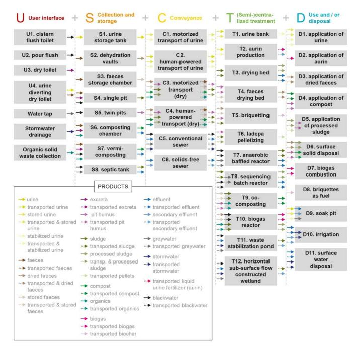
Figure 5.2:Overview of the 41 technologies in this study used to generate sanitation systems and to quantify their substance flows grouped by functional group. Each technology is defined by its name, possible input and output products, and how these products relate to each other (e.g. 'OR' for either one or another, 'AND' if they always arise jointly. Taken from Spuhler et al., (2020c).
