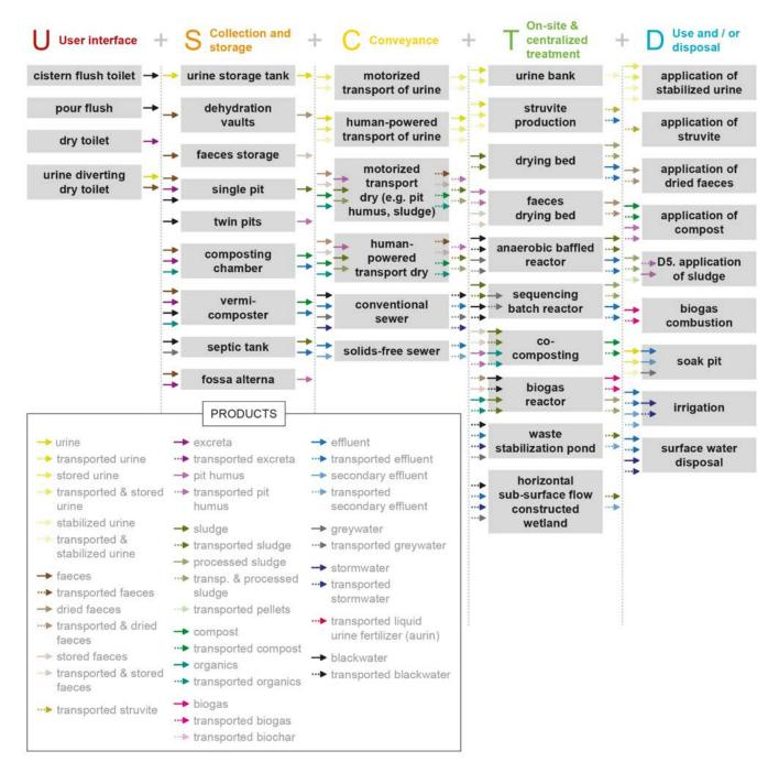
Figure 6.4: Potential technologies tested with Santiago in Arba Minch. Each box represented a technologies and the arrow indicate the input and output products used to check their compatibility. A detailed description for each technology is provided in the technology library at ERIC: https://doi.org/10.25678/0000ss.
