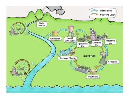
Figure 1.4: Sustainable sanitation addresses the entire cycle from the toilet to the collection, treatment, and reuse, and closes water and nutrient cycles in order to protect natural resources and people downstream. Picture: (Conradin et al., 2010).
