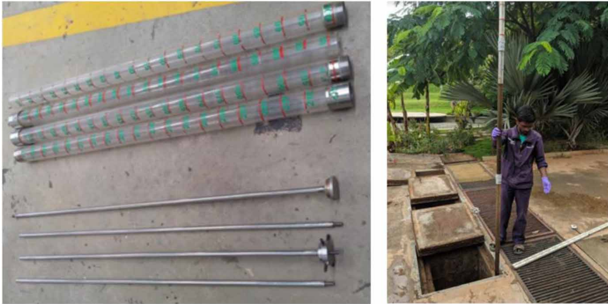
Figure 1 | Core sampler used for measuring the height of the sludge blanket and the total height of faecal sludge.
