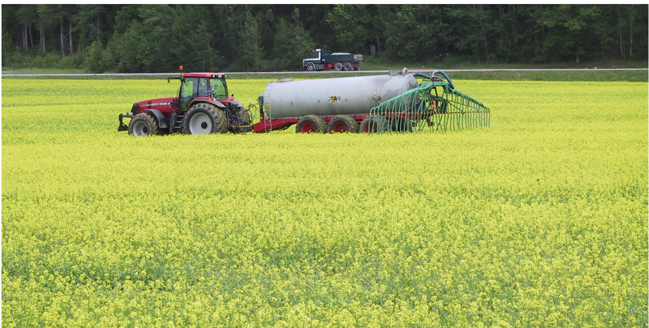
Figure 5. Brassica rapa fields fertilised with stored urine applied with a trailing hose spreader.
