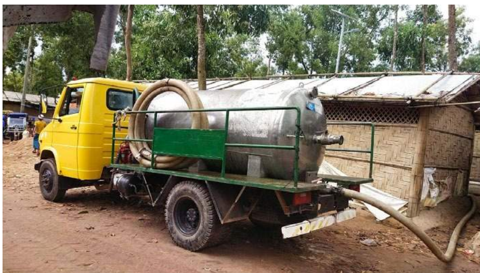
Figure 10: Example of VacTug
