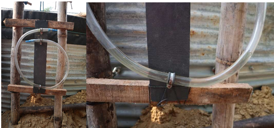
Picture 8a+b: Pressure regulator and close up on oil filling
