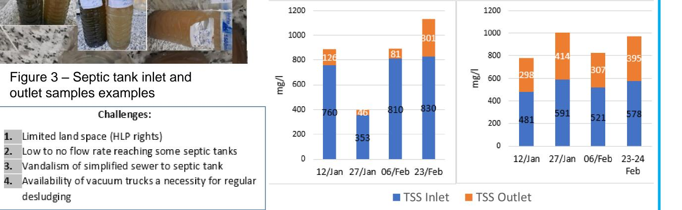
Septic tanks achieve high solids removal 70-90%, 50-80% COD and BOD of about 30-50%. However, effluent from septic tank requires further treatment since it partially removes BOD load and does not kill pathogens or remove nutrients. Reuse of the effluent without treatment is discouraged. Depending with the desired end use or receiving waters, septic tanks can be operated in combination with waste stabilization ponds, constructed wetlands, UASB and others.
