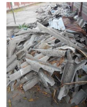
Example of suspected asbestos containing material among debris from Tropical Cyclone Idai, Mozambique.
