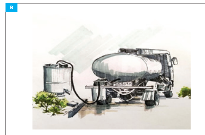
Figure 3: (A) A sketch of a purpose-built water distribution truck (B) A sketch of a purpose-built truck discharging water at a fixed storage tank. (Adapted from WHO-WEDC, 2013)
