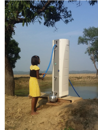
Figure 7: Manual ultrafiltration in operation (Source: www.villagepump.org )
