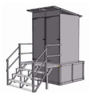
The cost of a double cubicle raised latrine is £450 and supplied through the <u>Oxfam procurement</u> <u>centre</u> in multiples of 6. Each twin latrine has a holding tank of 2m3.
