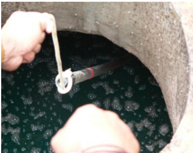
FIGURE 20: Liquid level can be monitored by observing level in sampling pipes. [24]
