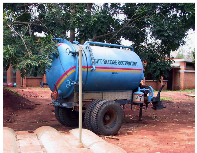
FIGURE 21: Cleaning the pipes with a brush (left) and desludging by vacuum truck (right). [25]
