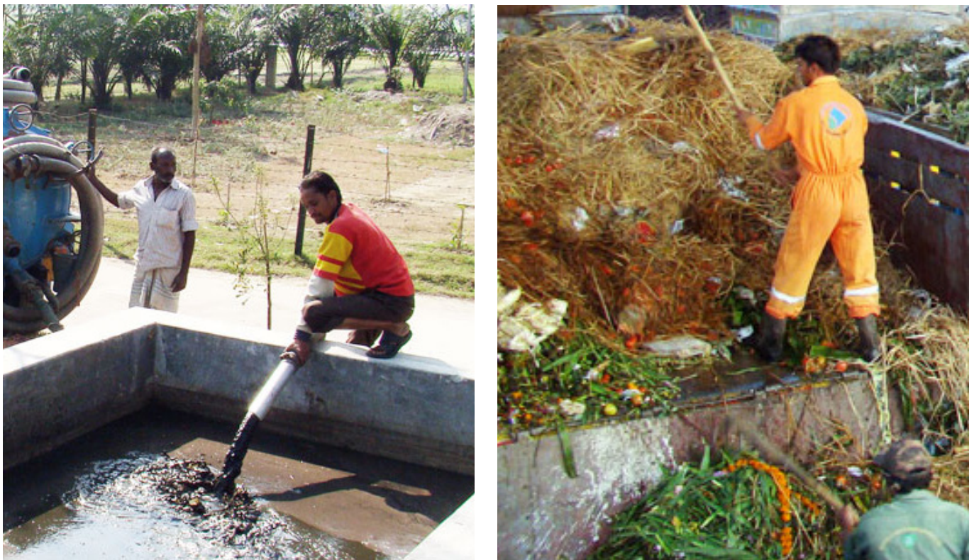
FIGURE 41: Co-composting improves the C/N ratio, combining faecal sludge (left) with organic waste (right). [36]
