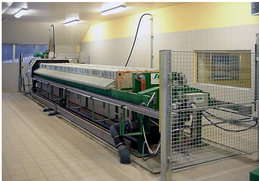
FIGURE 34: Press filter (top), detail of the side of a press filter (center), and cakes produced by press filters (bottom). [30]
