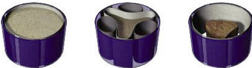
FIGURE 14: Working principle of the porous tubes: filled with sludge (left), air pressured filtration (center) and final press cake (right). [9]
