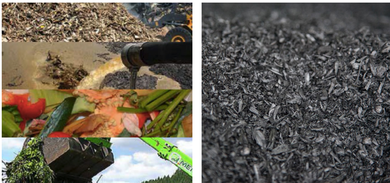
FIGURE 44: Pyrolysis uses biogenic residues as input (left) to obtain valuable liquids, fuel gas, and binding biochar as outputs (right). [38]
