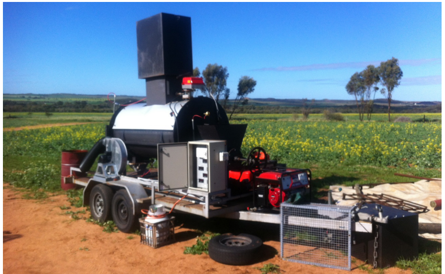
FIGURE 48: Mobile sludge pyrolysis systems. [42]
