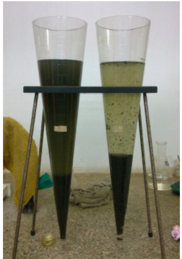
FIGURE 7: Faecal sludge from lined pit latrines (left) and from septic tanks (right).
