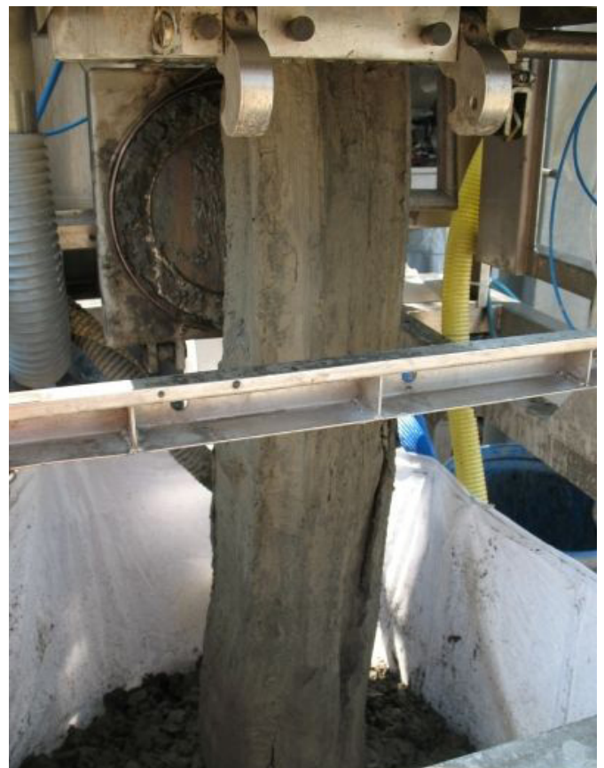
FIGURE 13: Press cake after tube compression. [8]
