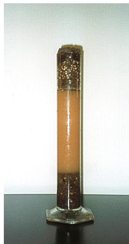
FIGURE 10: Example of Organic Matter Separation in the Digester.
