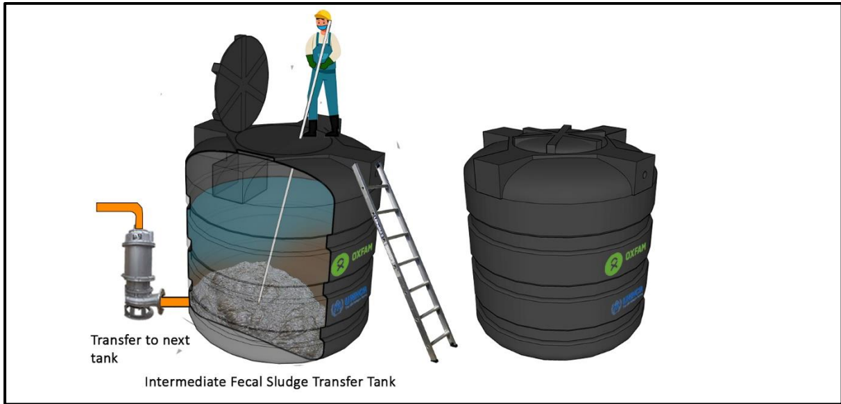
FIGURE 9: MANUAL STIRRING INSIDE PLASTIC TANK WHILE PUMPING TO NEXT TRANSFER STATION
