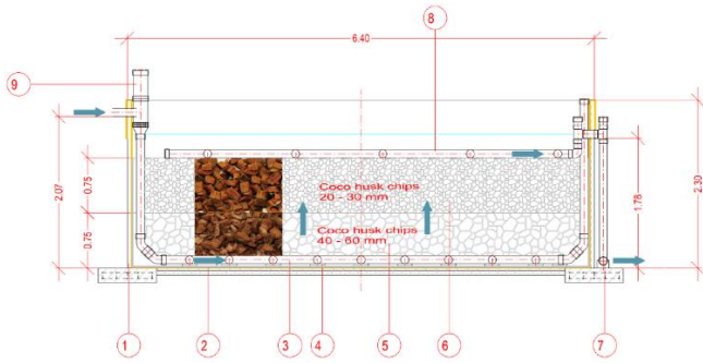
Initial Upflow filter cross-section and image
